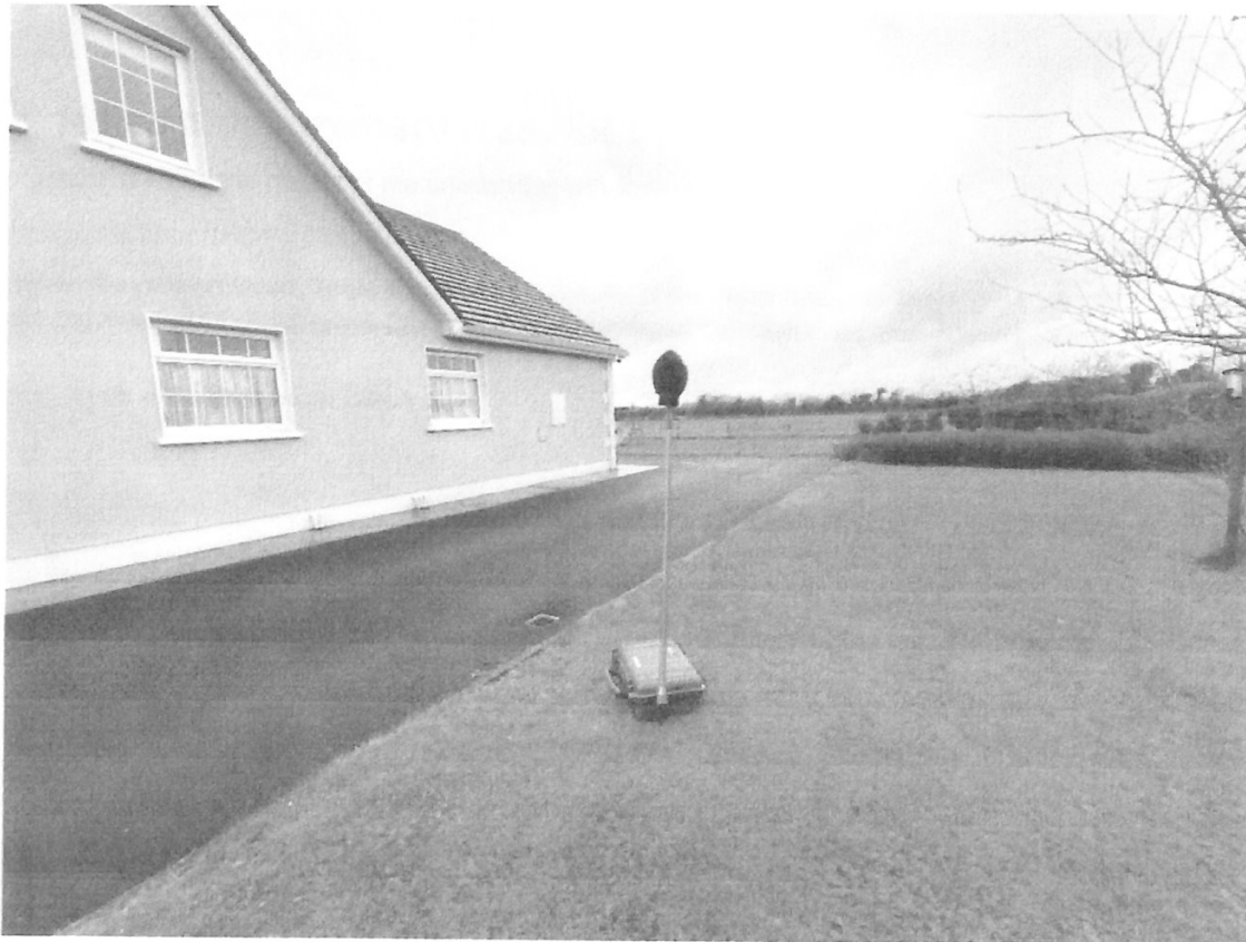
Figure 3: Noise Logger Setup
